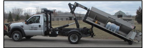
2008 Ford F550 with new Hook-lift System
