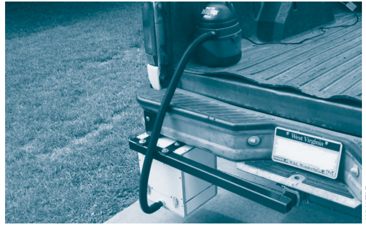
A mobile dust collector was used to determine the amount of dust released from the road when it was driven over.
