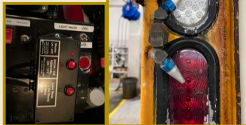
Tail Light Cleaner (Photos: Courtesy of City of Wyoming)
