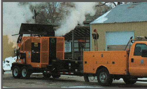
Millings from road project for recycling (top left) and asphalt recycler in operation (bottom left); Pavement in Traverse City prior to (top right) and after infrared patching (bottom right) (Photos: courtesy of City of Traverse City).
