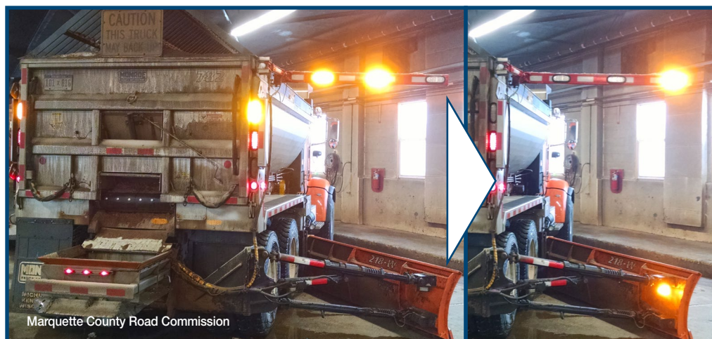
On top of adding hydraulic bars to increase the visibility of their wing plows, Marquette County Road Commission contacted local media to increase the public's awareness of wing plow use. One of these communications, a video and interview done by a local news channel, can be watched at https://youtube.com/watch?v=9OW_qQx2kic
