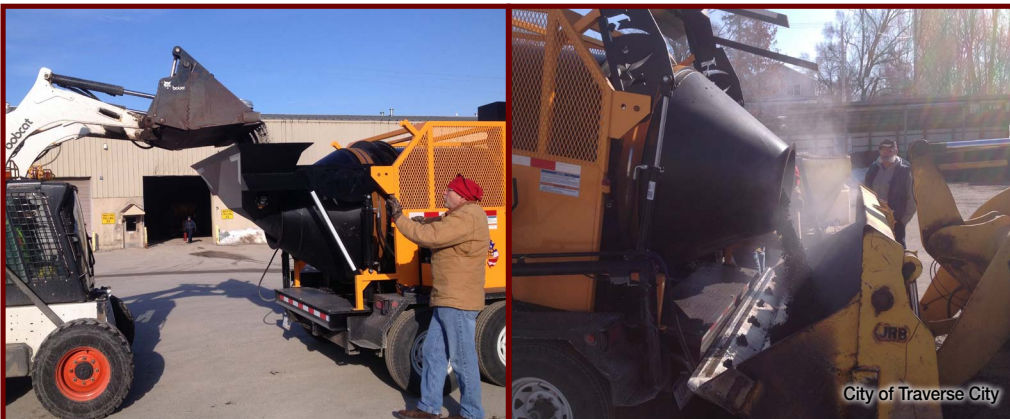
City of Traverse City recently purchased an asphalt recycler (above) to compliment their infrared recycler. This ensures that material lost from potholes can be more easily replaced during the infrared recycling process.
