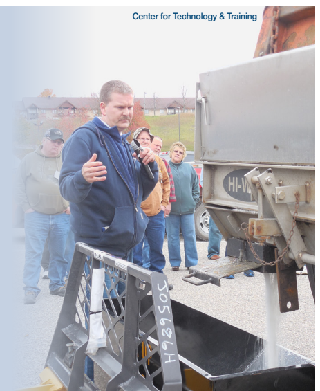
City of Farmington Hills' Bryan Pickworth demonstrates salt spreader calibration at the 2013 Winter Ops conference.
