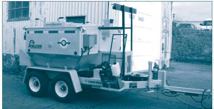
City of Pittsfield's asphalt reclaiming hot box.
