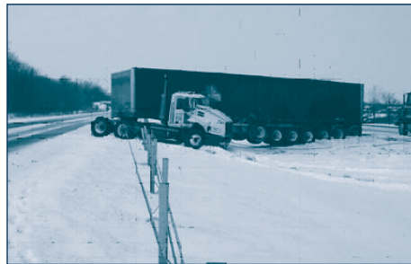
A cable barrier in the median prevented this tractor trailer from crossing the median and entering an opposing lane of traffic on a Michigan highway.
