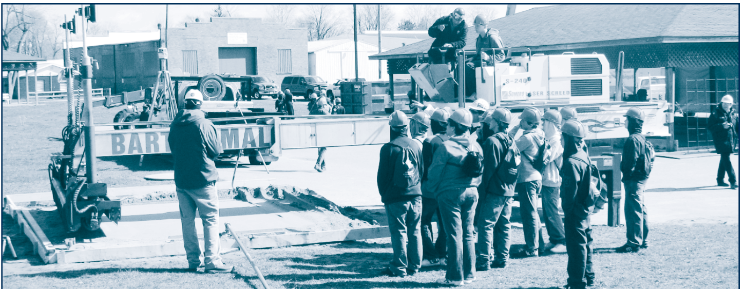
Students experimented with a Laser Screed®, a high-tech material placement machine which was provided by Barton Mallow.
