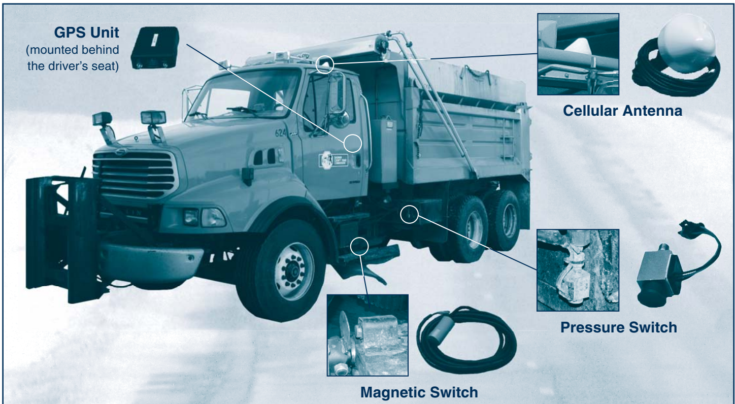
Truck-mounted components of Saginaw County Road Commission's Automatic Vehicle Location (AVL) system.
